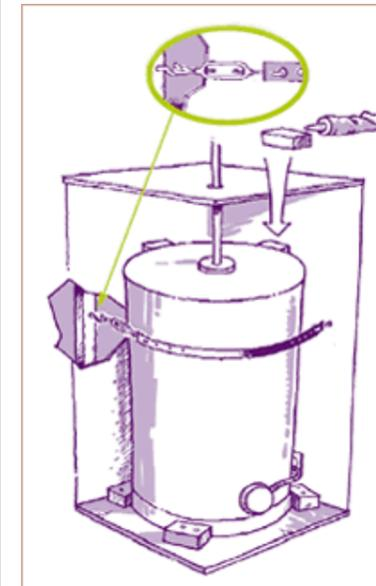
Even small shakes can cause hot water cylinders to rock enough to crack pipes, often causing expensive and messy water damage. In larger earthquakes the cylinder can tip over completely, with hot water becoming a hazard. Both can deprive you of your largest source of drinking water after a disaster. Securing a hot water cylinder is surprisingly easy.
