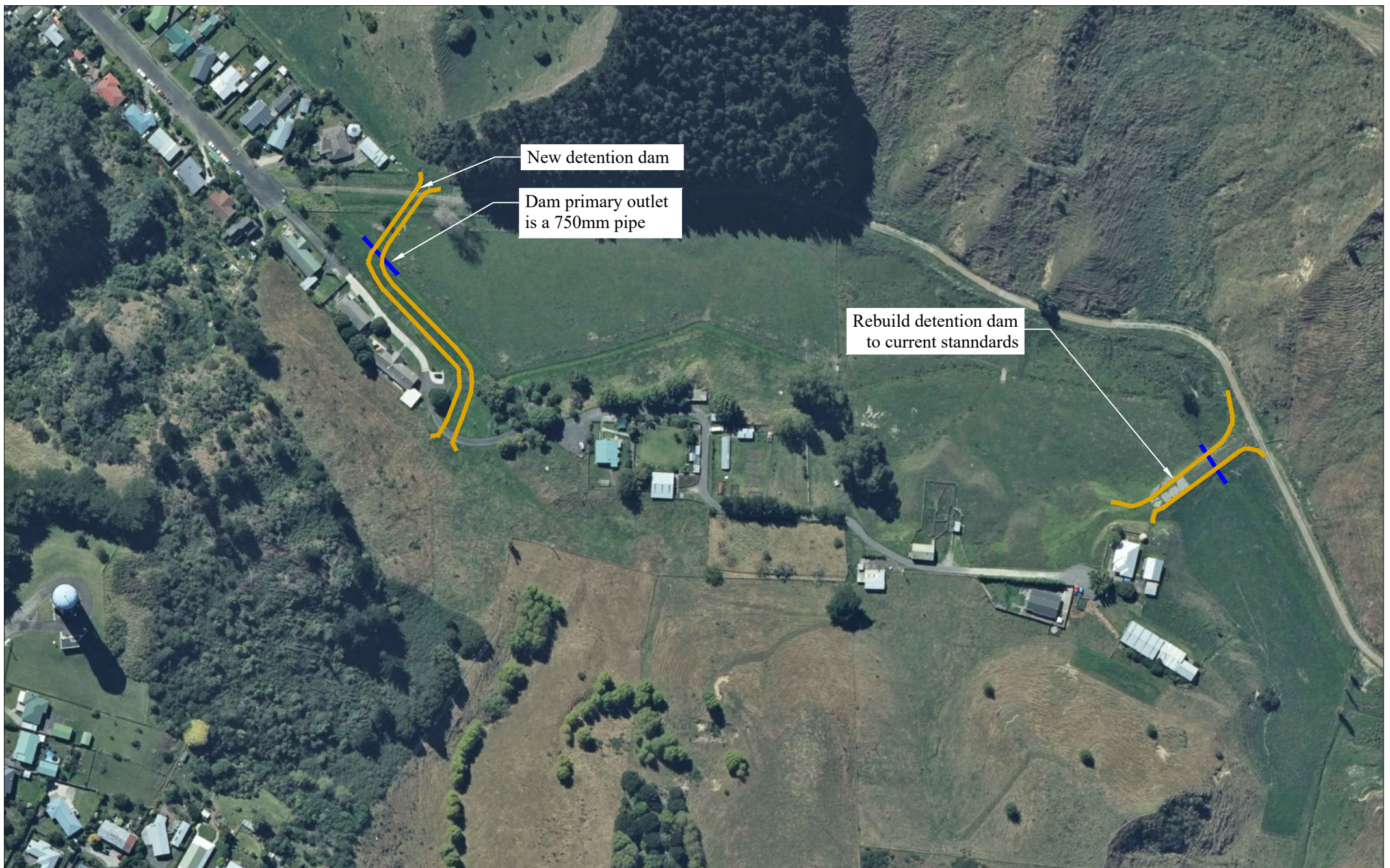
Option 4 - Detention Dam End of Turoa Road Scale 1:2500 (A4)
