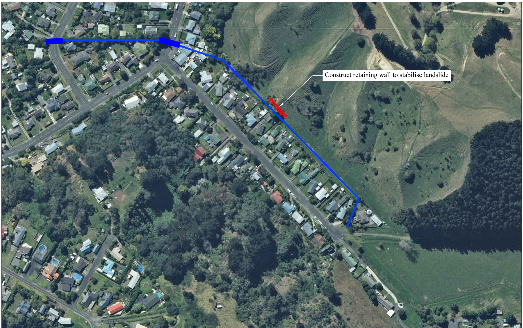
Option 1 - Construct Retaining Wall to Stabilise Slip Scale 1:2500 (A4)
