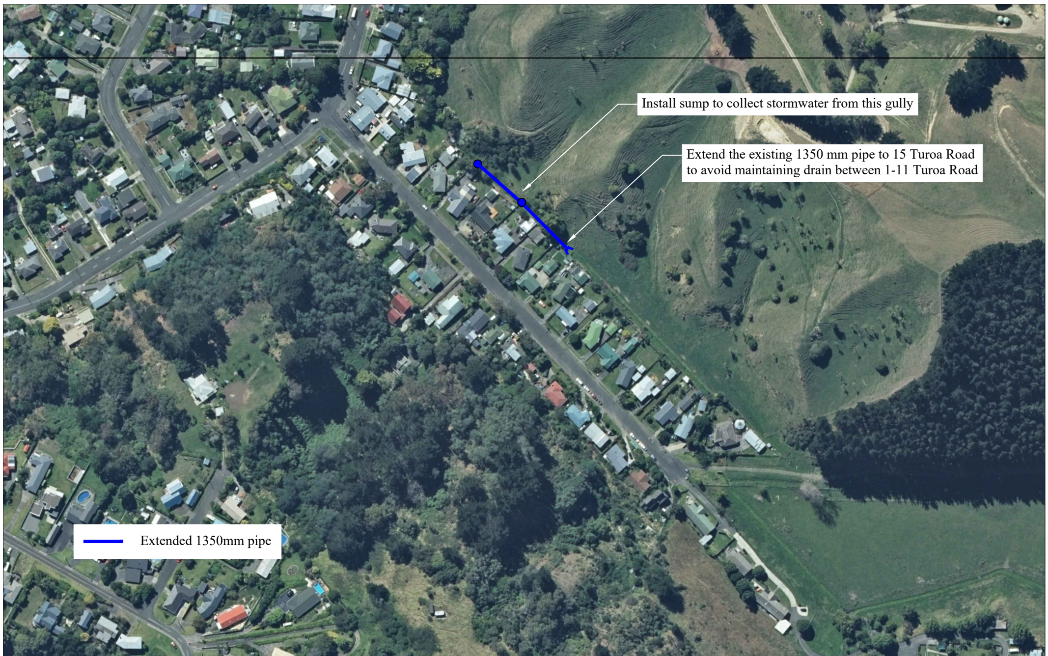
Option 3 - Partially Extend Pipe to 15 Turoa Road Scale 1:2500 (A4)
