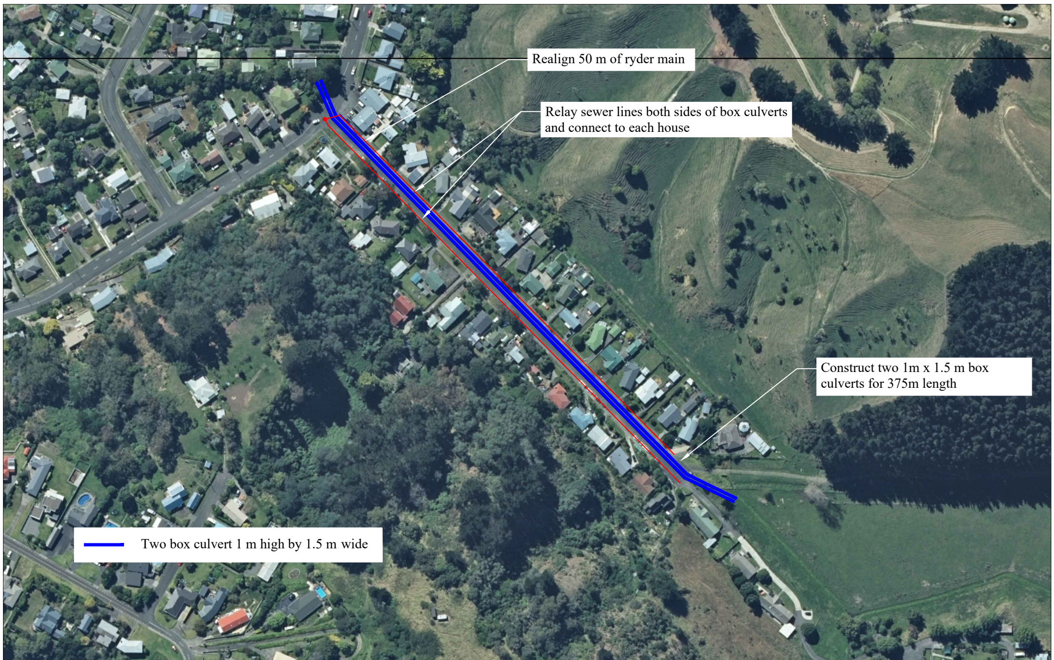
Option 6 - Construct a Large Overflow Pipe along Turoa Road Scale 1:2500 (A4)
