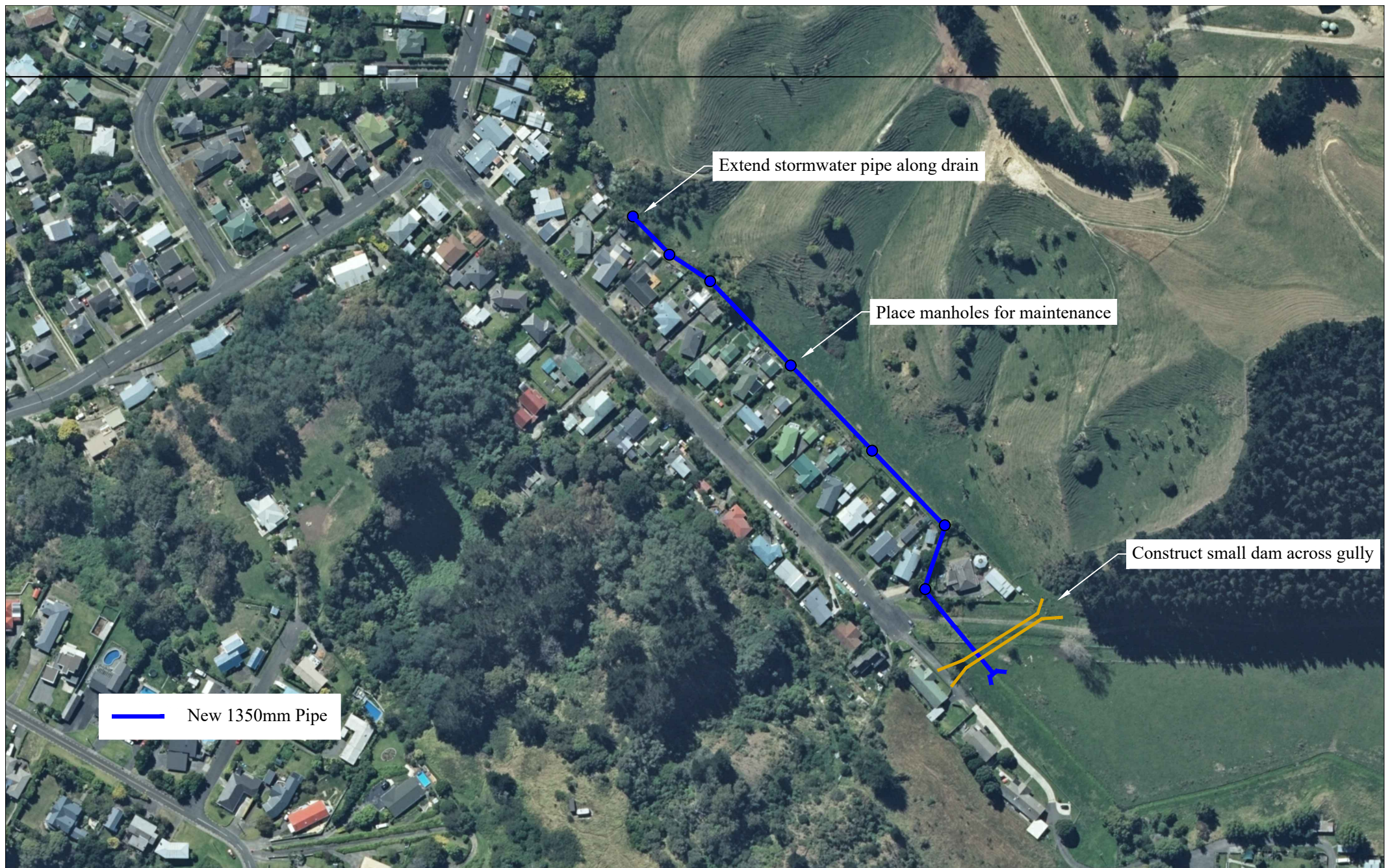
Option 7 - Extend Stormwater Pipe up Turoa Road Drain Scale 1:2500 (A4)
