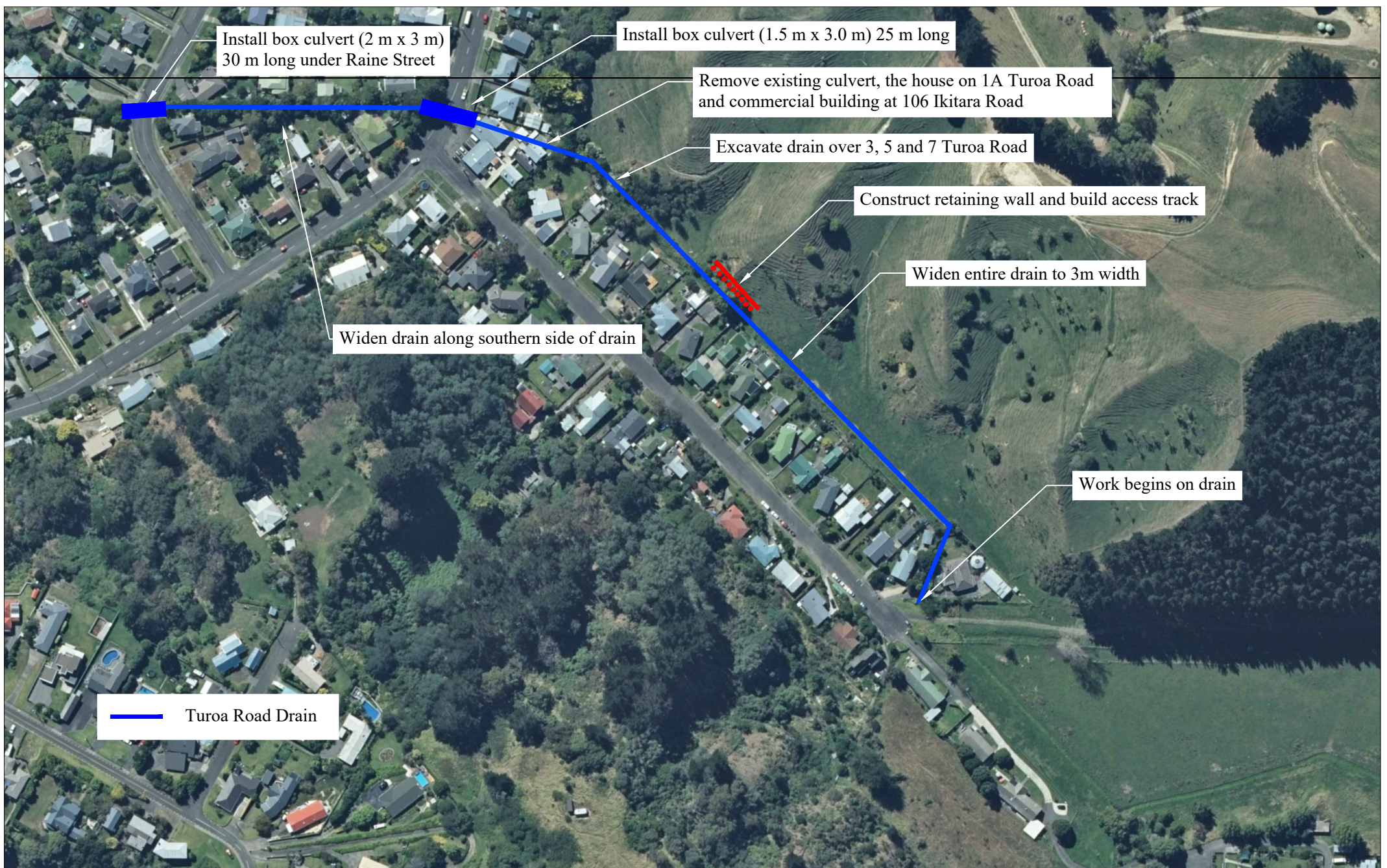
Option 5 - Widen Drain and Increase Size of Culverts Scale 1:2500 (A4)
