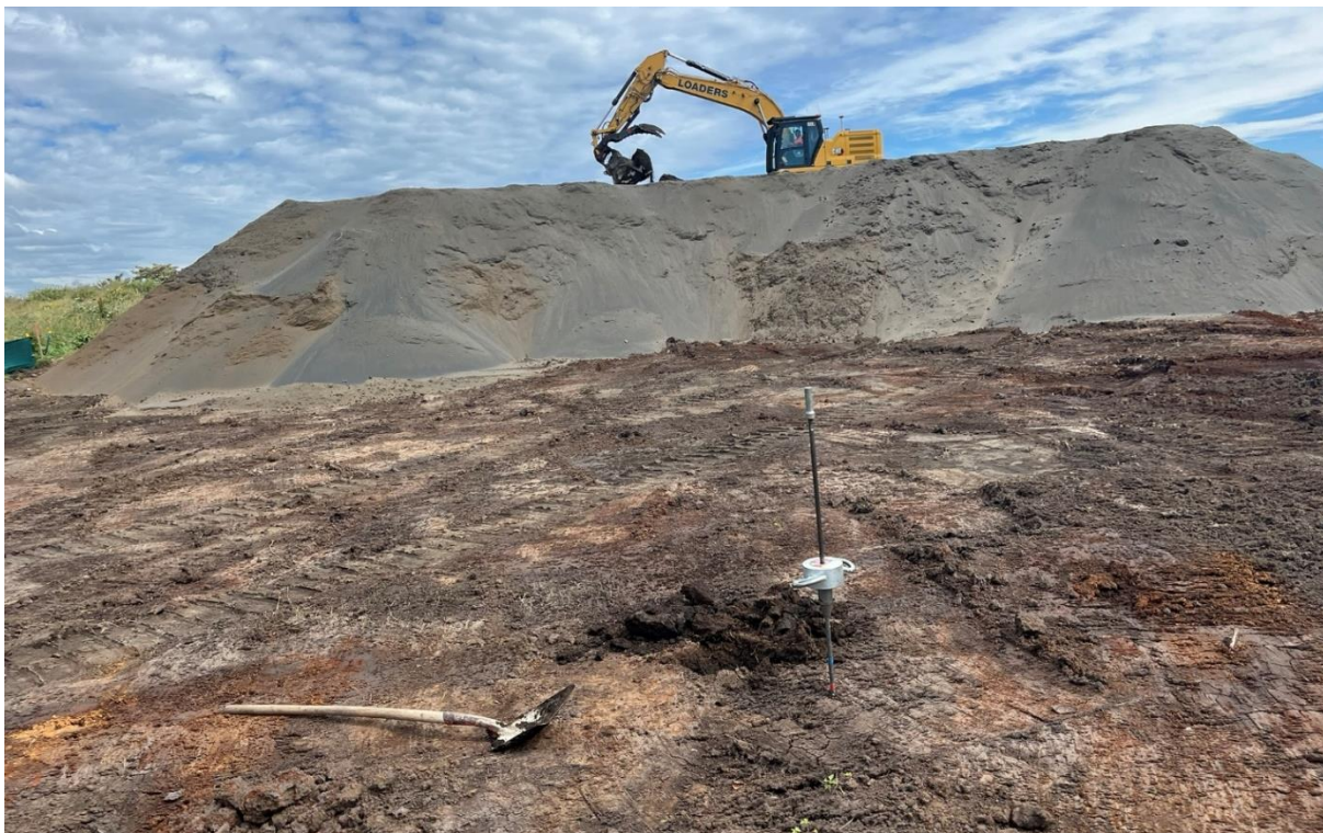
Figure 12 : Fox Road cut to fill stockpile. Scala Penetrometer testing of exposed subgrade.
