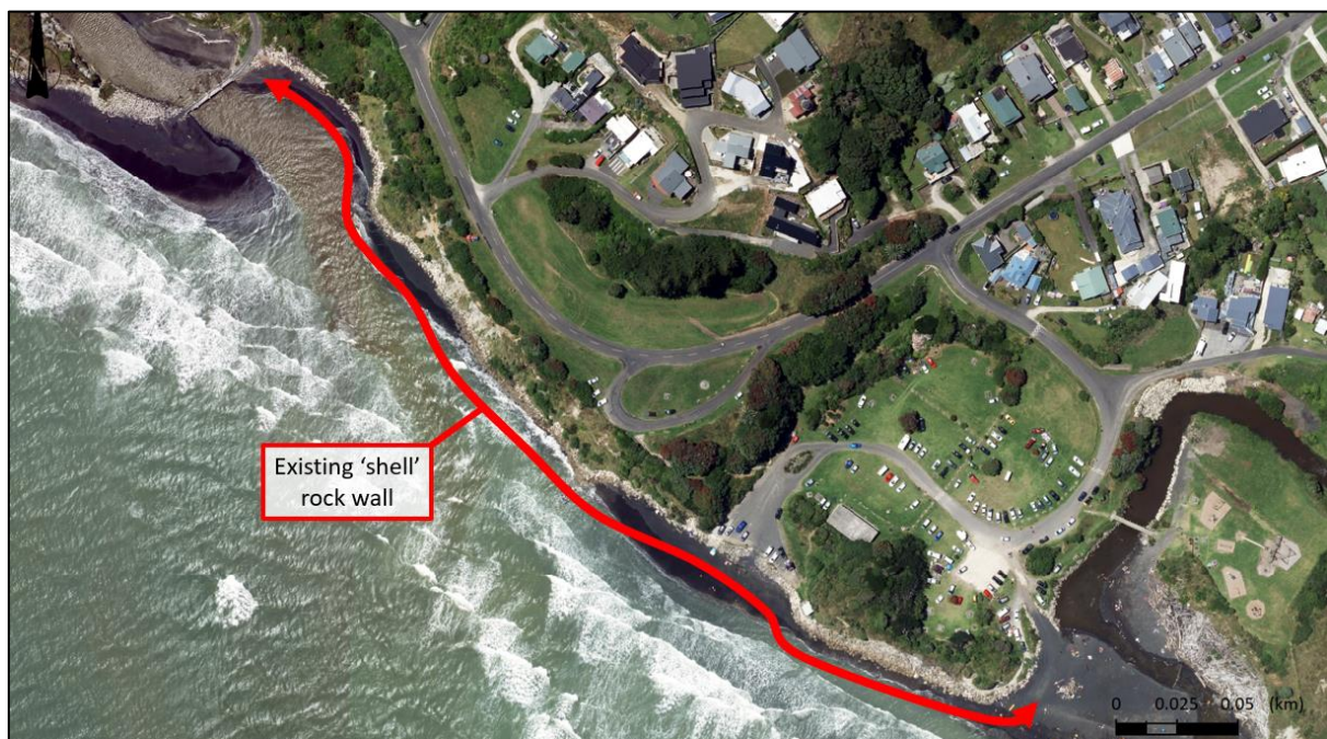
Figure 3.1: Extent of existing 'shell rock' revetment wall between the Kai Iwi and Mowhanau stream mouths
