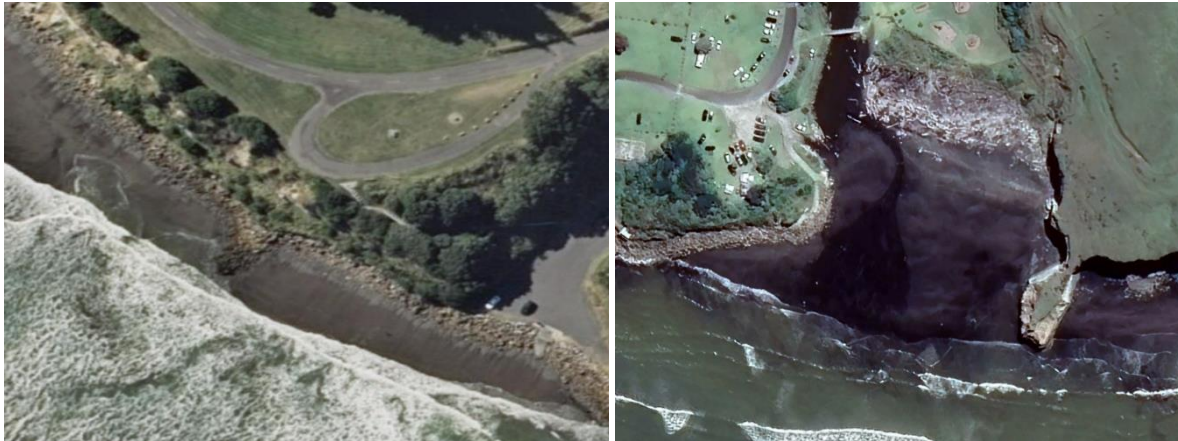
Photograph 3.7: Examples of an existing manmade (left) groyne at Kai Iwi with no appreciable sand accumulation on the updrift (north) side evident and a pocket beach (Mowhanau Beach) adjacent to a natural headland (right)
