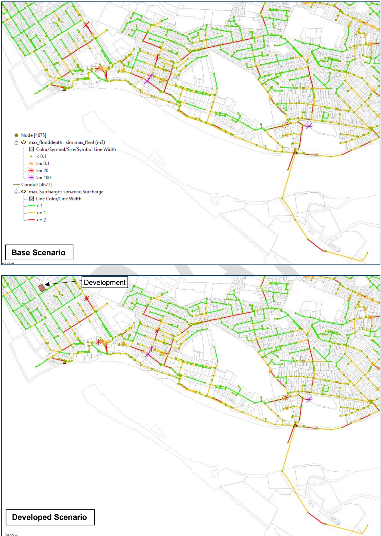
Figure 8 Network results showing manhole spilling for 1 in 1 year LoS event
