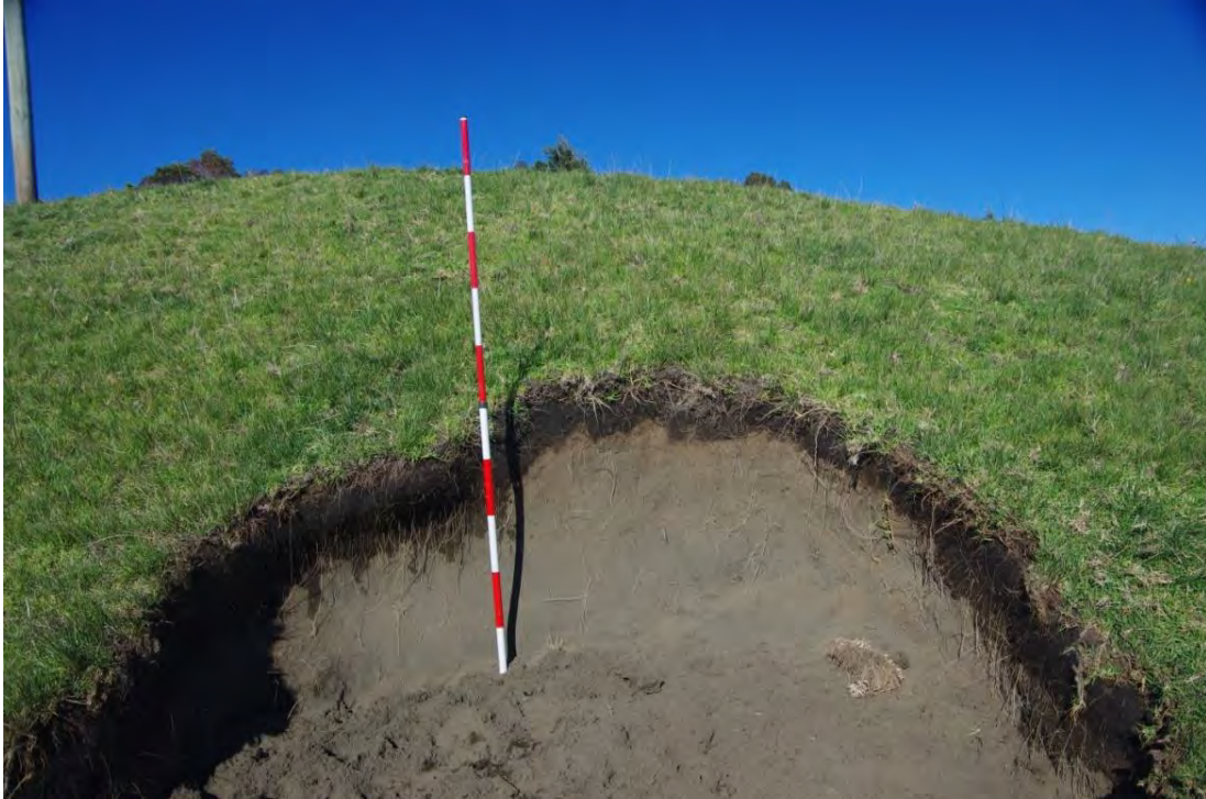
Figure 3: Section on a low sand dune near to Great North Road showing the natural dark topsoil that develops under grass, with a weakly developed grey-brown sand subsoil over lying clean lighter coloured sand.
