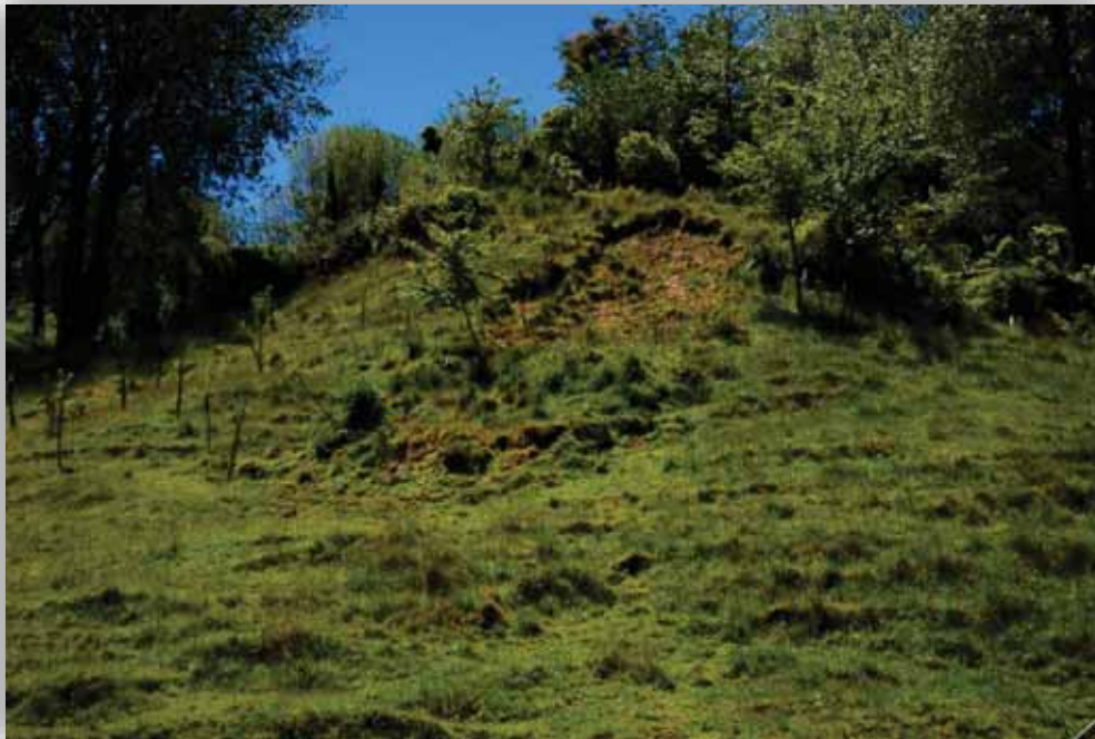
Illustration 2 Shallow slip in topsoil, near Paterson Street.
