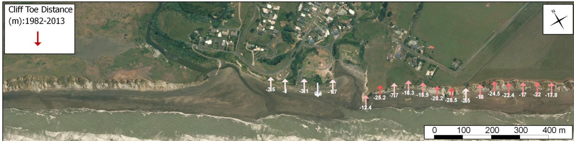
Figure 4.3. Cliff toe erosion rates for the 1982 to 2013 period.
