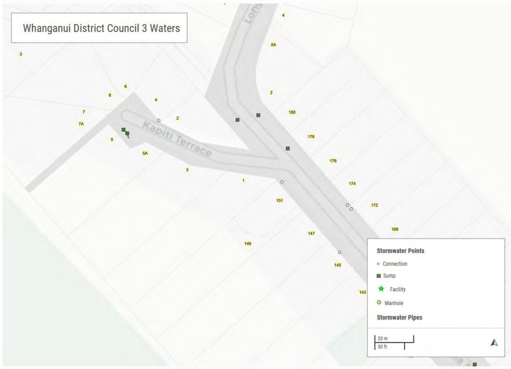
B. Location of existing stormwater sumps and pipes at the Kapiti Terrace end of Karaka Wetland. These are also proposed to be upgraded.
