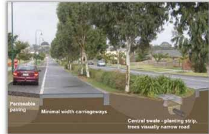
Figure 19 – Typical Swale Road Cross Section - North Shore
