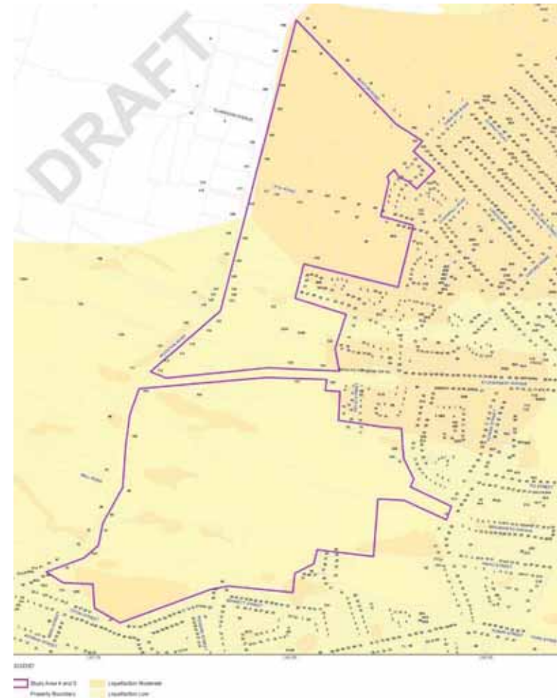
Figure 21 – Liquefaction Hazard Map
