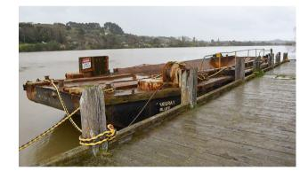
Whanganui Port's barge (pictured) has been moved to the city marina along Taupo Quay to "hibernate" for winter. The barge sustained damage at its port mooring recently due to ocean swells and surges so it will tie-up at the marina for shelter until repairs can be made. Please remember the barge is a commercial vessel and should not be boarded signs are displayed advising the community to please stay off the craft for safety reasons during its temporary mooring.
