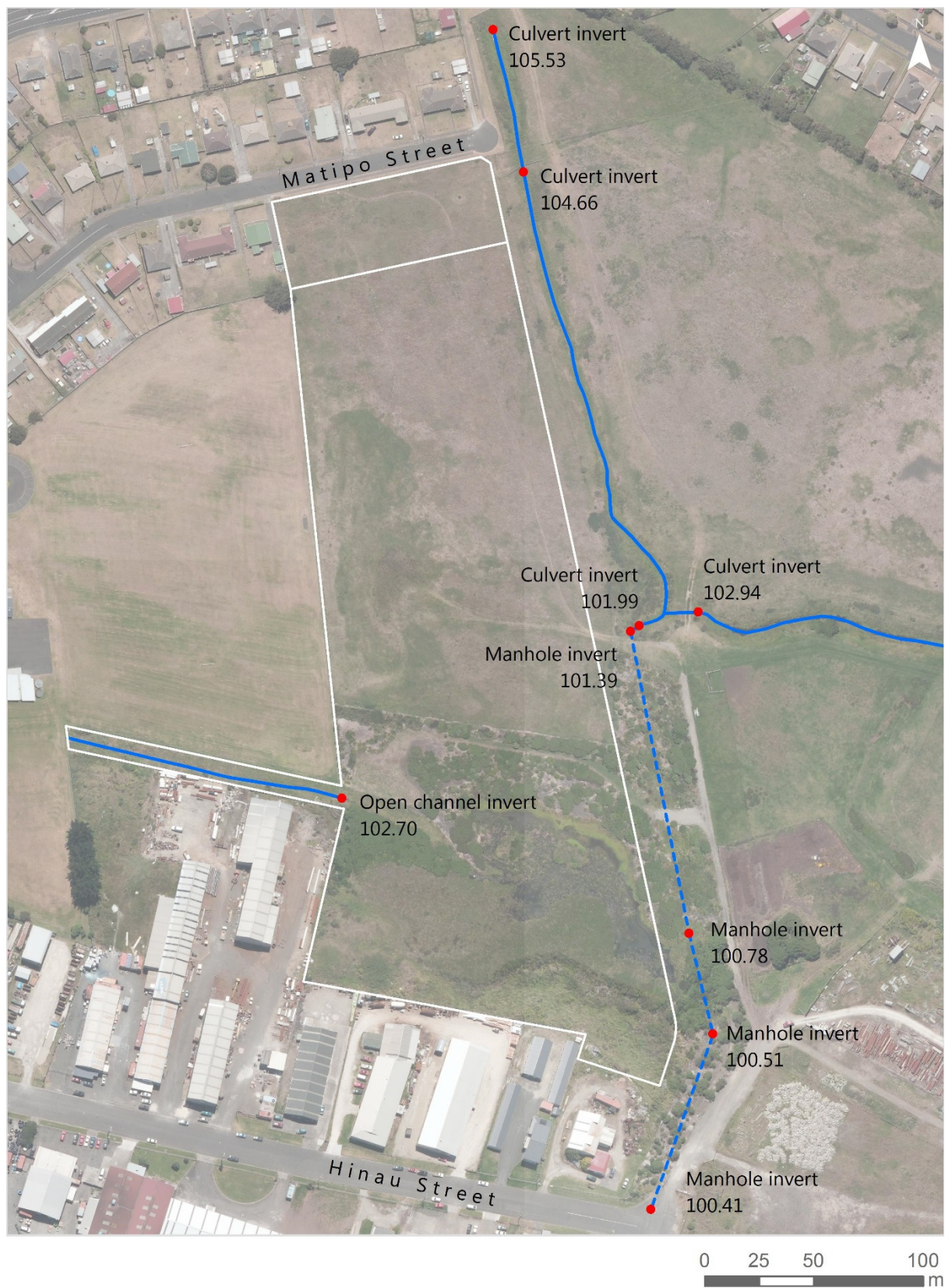
Figure 3. Surveyed channel, culvert and manhole inverts
