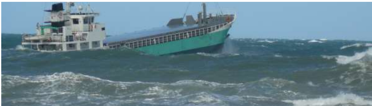
MV Anatoki pitching in a seaway showing reduction of draft fwd and increase in draft aft.
