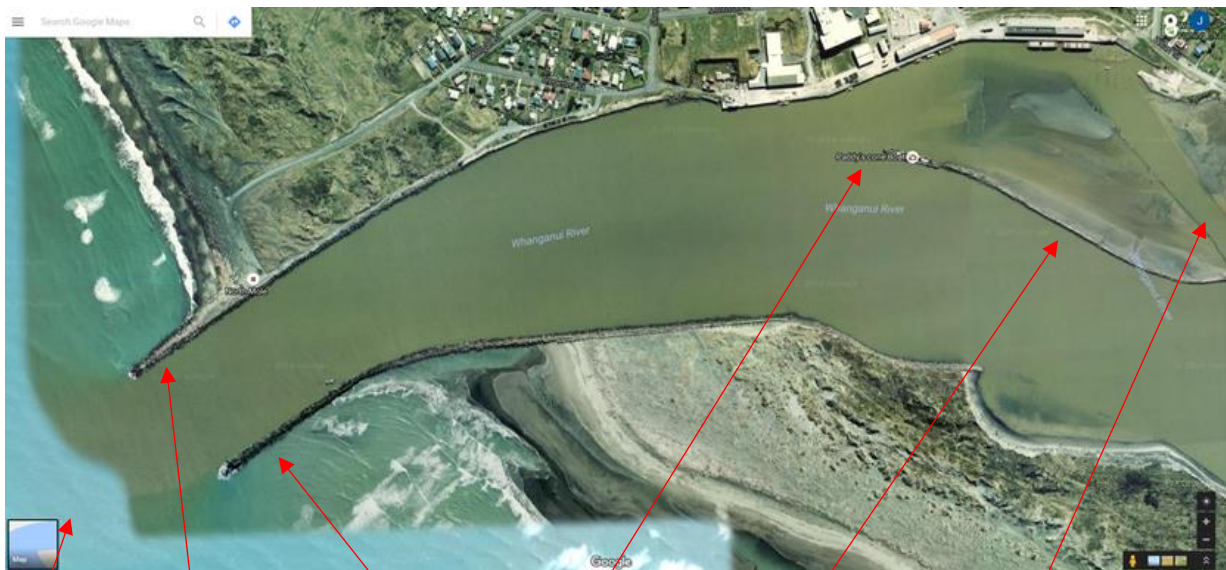
Bar North Mole South mole 'Te Anau' hulk Training wall Wall opening channel
