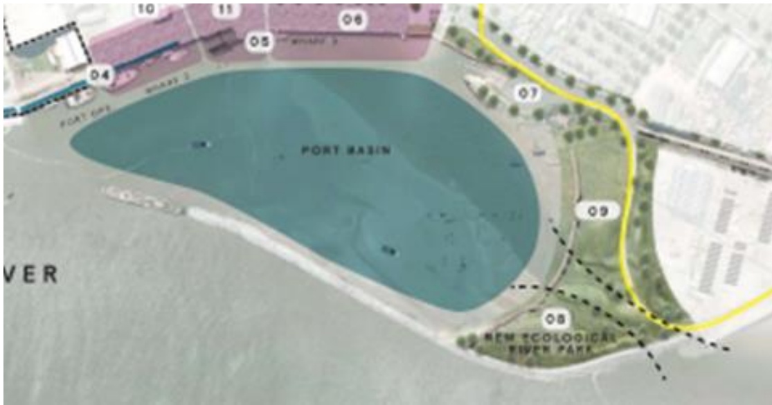
Figure 4. Indication of proposed redevelopment showing area of reclamation and closure of old channel.
