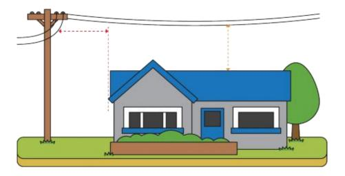
The distance between the building and the overhead power lines depends on the voltage and the type of line.
